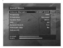
After setting the parameters of search, press the **OK** button to start channel search. Wait until the operation is completed. After finishing search operation, the result window will be displayed. You can delete the channels using the  $\triangle/\nabla/4/\triangleright$  and the **RED** button. To cancel deleting operation, press the **RED** button again. The screen also shows the number of the channels found and the transponder information.
